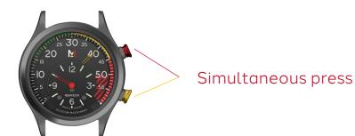
Validating minutes also resets seconds to O seconds. To set the seconds accurately, it is therefore necessary to validate the minutes at the moment when the minute of an official clock is exceeded.
