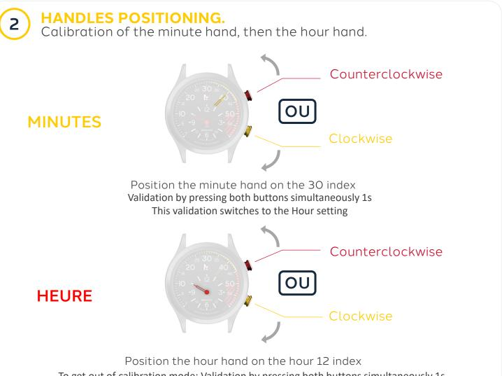
To get out of calibration mode: Validation by pressing both buttons simultaneously 1s
